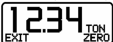
This will tell you the total amount of grease that has passed the meter since it was reset last time. Note that the smallest amount that will show is 1 kg (0.001 TON). To reset the total amount counter press ZERO (right button). To exit the menu press EXIT (left button).
