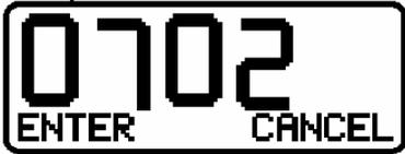
Press ENTER (left button) to accept and save the new calibration, or CANCEL (right button) to cancel the changes and return to the old calibration factor.
