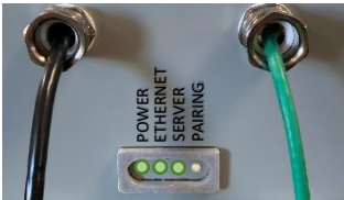
Figure 10 Sensei Gateway status lights. The Power, Ethernet, and Server lights will all turn green if the gateway is configured properly.
