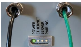
Figure 6 There are two ports on the bottom of the enclosure used to pass power and data into the enclosure. In this figure Ex rated cable glands are being used.
