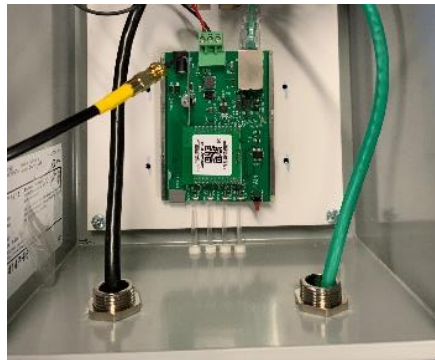
Figure 15 Press the red pairing button on the Sensei Gateway to add Sensei Repeaters to the network.
