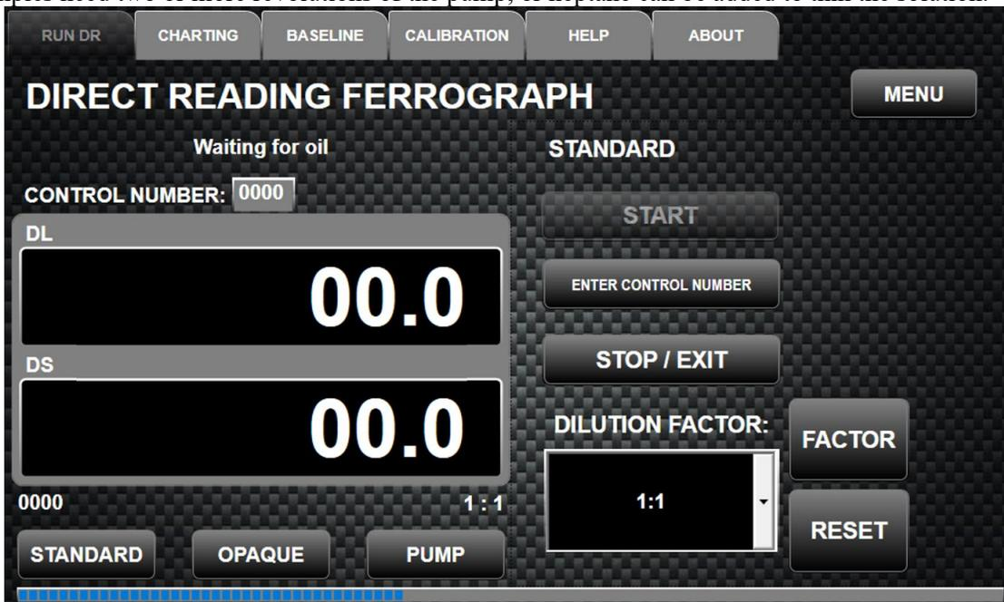
7. As oil flows through the precipitator tube, the Display Messages will change through the following phrases, colored white, letting the operator know the progression of the test.
