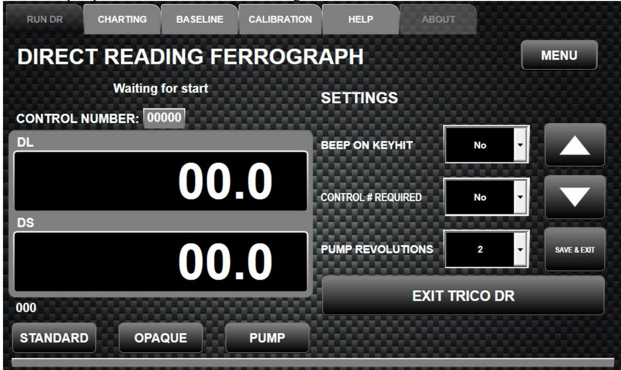
Selections can be made by touching the desired setting pull down and hitting the up or down arrows to the side to scroll through the selections. After all changes are made press the SAVE & EXIT button to set the new selections and then exit to exit out of the menu. Default settings are, Beep on key hit: No, Control number required: No, Pump revolutions: 2.
