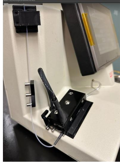
4. Place the end of the capillary tube in the oil sample in the vial holder until it touches the bottom of the sample vial and press the tubing into the spring at the top of the sample vial holder to hold the tubing in place.
