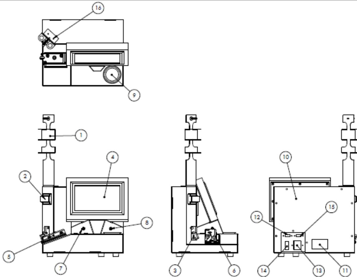
This section introduces the user to the major components of the DR-7 Direct Reading Ferrograph Instrument. The following subparagraphs discuss the major components, their location, and the nomenclature for each item on the DR-7 Direct Reading Ferrograph Instrument shown above.
