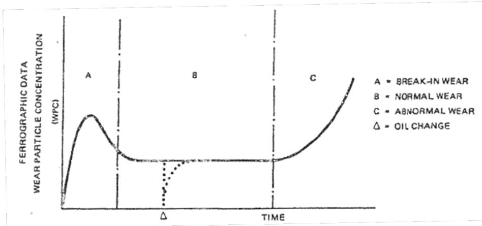
Figure 8.1A Typical Large Particle Profile
