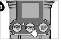
Press the POWER button for 2 seconds to turn the unit on.
