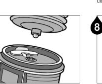
Purge the grease pouch until grease comes out of the tip.
