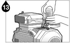
Install the Streamliner M unit on the lube point. When the selected dispensing period has completed, replace the unit with the Service Pack according to step #3~7.
