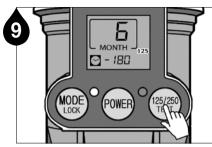
Select the appropriate grease pouch capacity by pressing the 125/250/TEST button.
