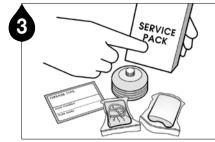
Check the grease pouch capacity and the service pack items (battery pack, grease pouch & dust cover).
