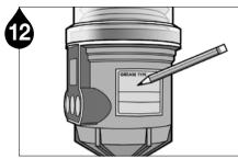
Note the installation date and the scheduled completion date of lube cycle on the lubricator using the label provided in the Service Pack for maintenance purposes.
