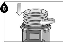
Carefully screw the grease pouch in by turning clockwise. Do not over tighten.
