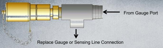
Hose, tubing or the pressure gauge from the main system pressure port is removed and replaced by a hydraulic tee and appropriate hardware. Sample port is installed so that the flow of the fluid is directed at the Sample port.
