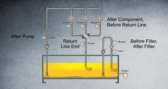
Installation of forced lubrication system require the sample port installed after the component.
