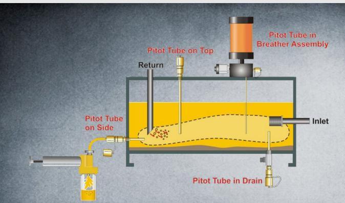
Installation in a hydraulic reservoir require the pitot tube to be installed at approximately ½ the height of the liquid level in a turbulent area. Watch for baffles internally.
