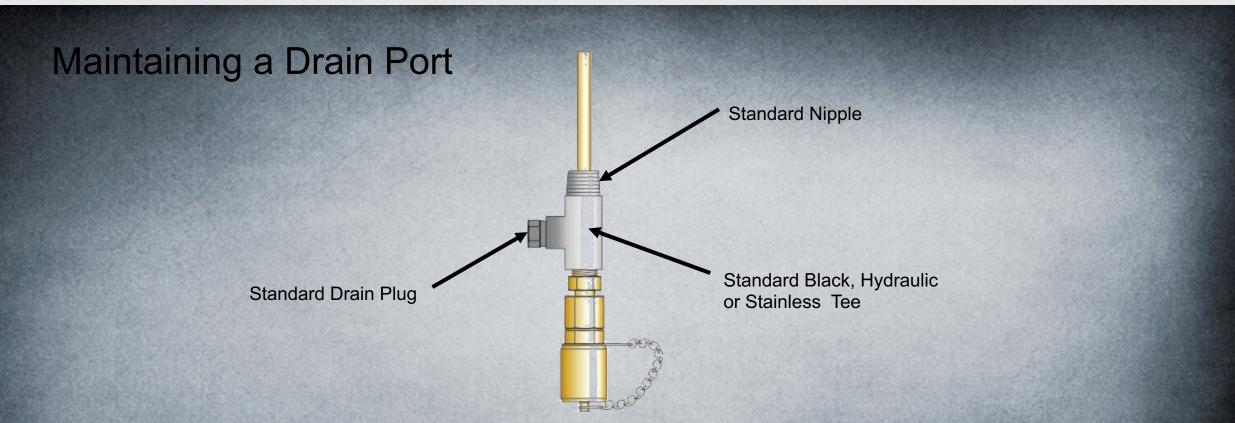
This method does not require the pitot tube to be removed to drain the lubricant.
