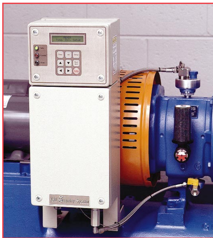
Figure 1. Monitoring the Lubricant in a Process Pump
