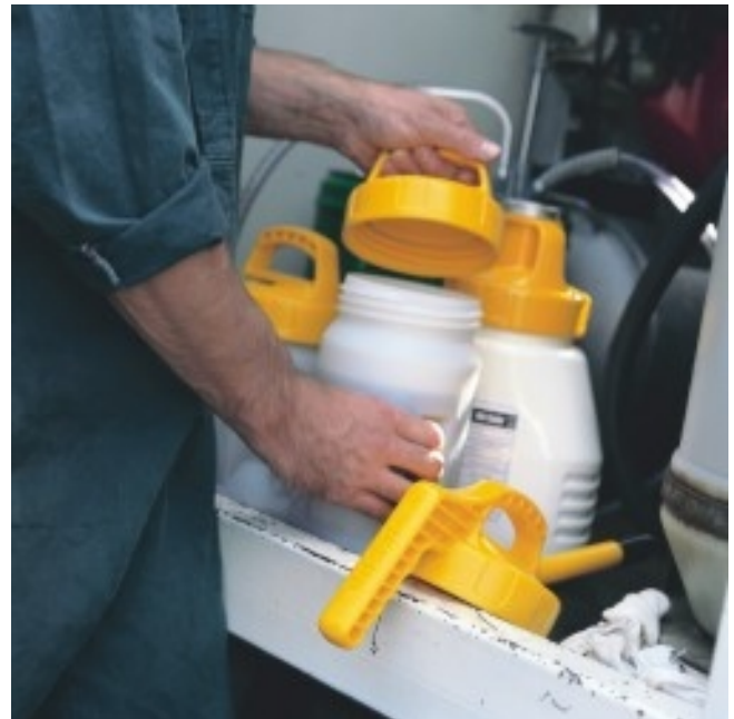
Figure 10. Oil Transfer Equipment.
