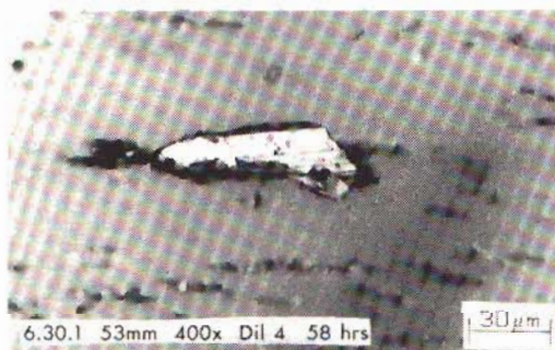
Fig. 14—Gear Set 6—Severe sliding wear
