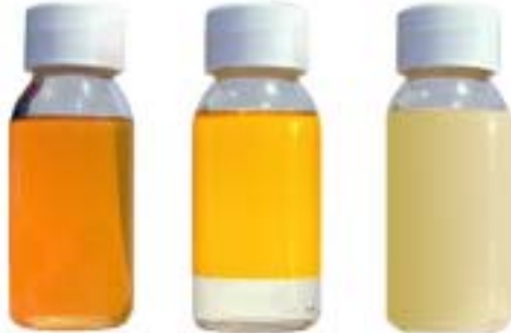
Figure 2. Dissolved, Free, and Emulsified Water
