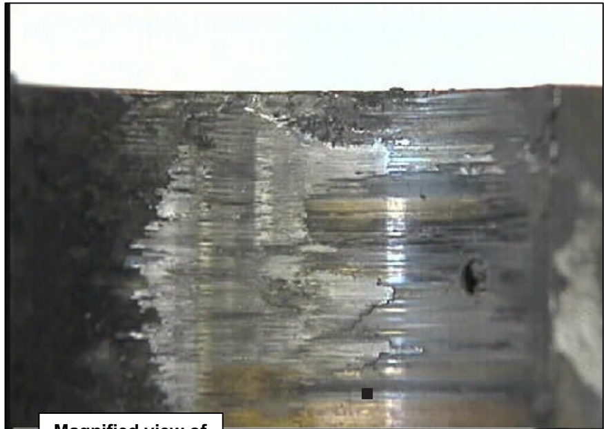
Magnified view of bearing surface
