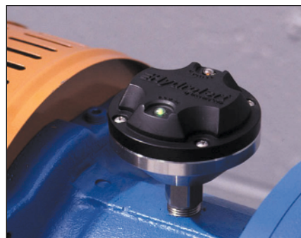
Photo 1. Oil contamination monitor
