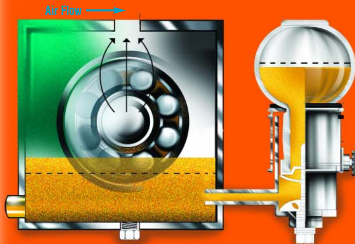
Figure 5. Pressure Differential from Air Flow
