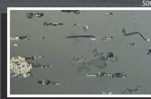
steel particles, cutting wear
